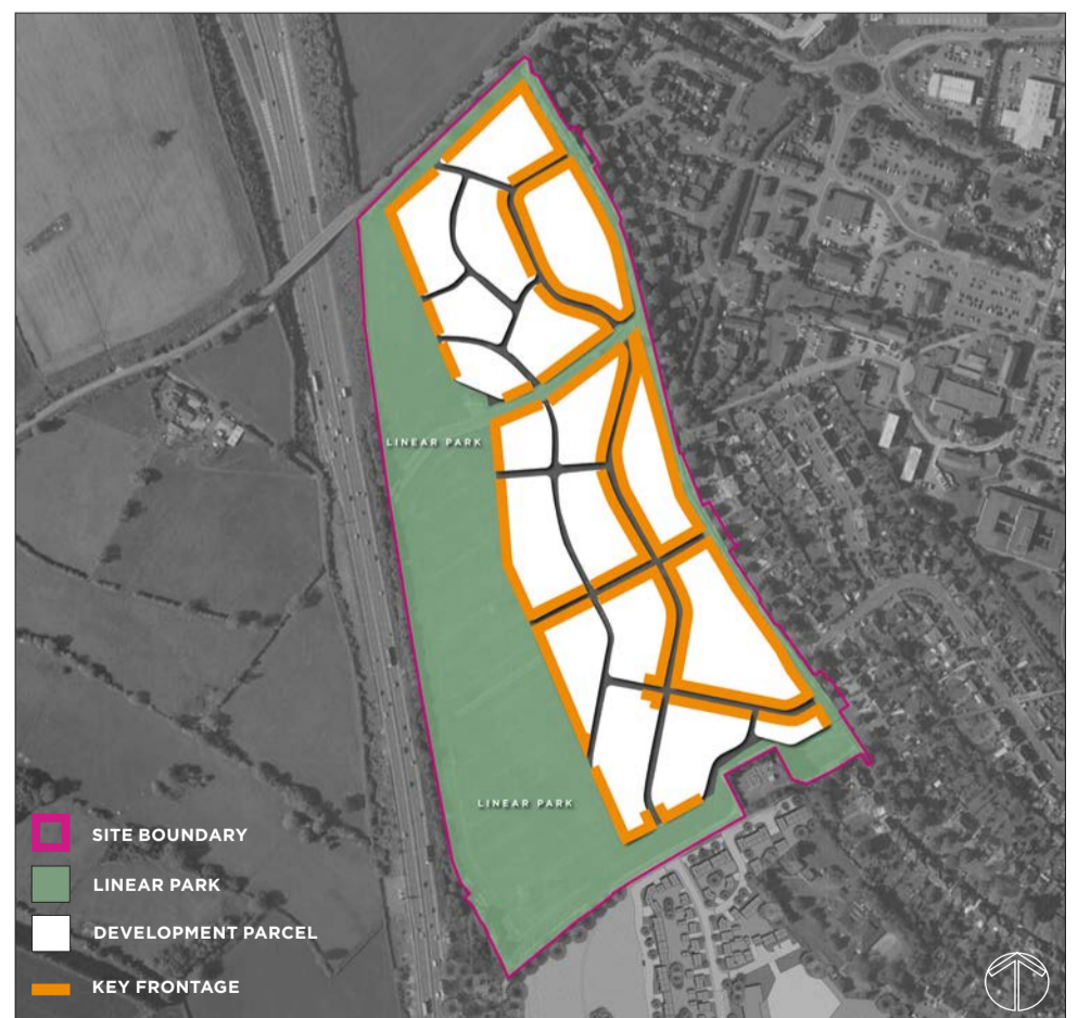
RATIONALE 4 - THE STREET ARRANGEMENT PROVIDES A SERIES OF DEVELOPMENT PARCELS WITH KEY FRONTAGE ALONG GIPSY LANE, THE SPINE STREET AND FACING AREAS OF PUBLIC OPEN SPACE
