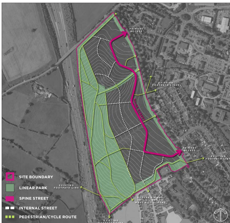
RATIONALE 3 - THE STREET NETWORK IS DESIGNED FOLLOW THE SITE'S CONTOURS. A SPINE STREET RUNS THROUGH THE CORE OF THE DEVELOPABLE AREA AND A NETWORK OF FOOTPATHS AND CYCLE ROUTES CRISS-CROSS THE LINEAR PARK
